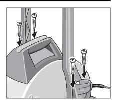
**Step 2** Insert each of the four long screws and tighten.
